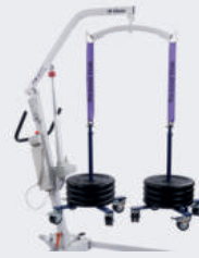
suspended condition (Test with a 185 kg hoist)
